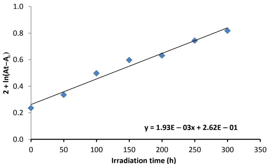
Fig.(5): Changes in  $\ln(A_t - A_\infty)$  for PVC film containing  $Bu_2SnL_2$  with irradiation time.
