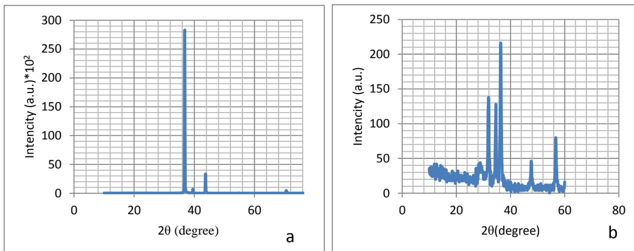
**Fig.(2): XRD spectra of (a) Zn target as a pellet and (b) ZnO target as a nano particles thin film prepared by electrophoretic deposition (EPD).**
