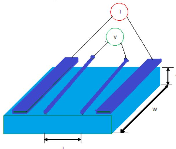
Figure 2. Schematically the membrane electrical contacts in the cell [8].
