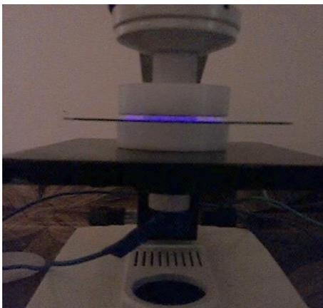
**Fig.(1):** Photographic picture of DBD system used to treat of films.
