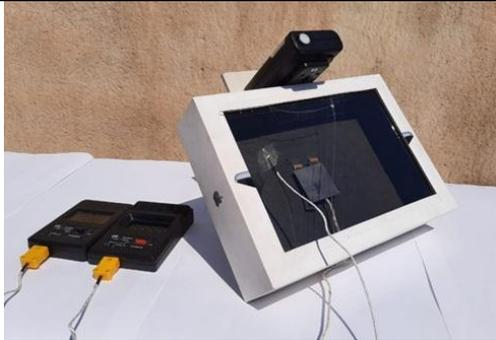
**Figure 3.** The flat-plate collector system used for the measurement of the solar-thermal characteristics.
