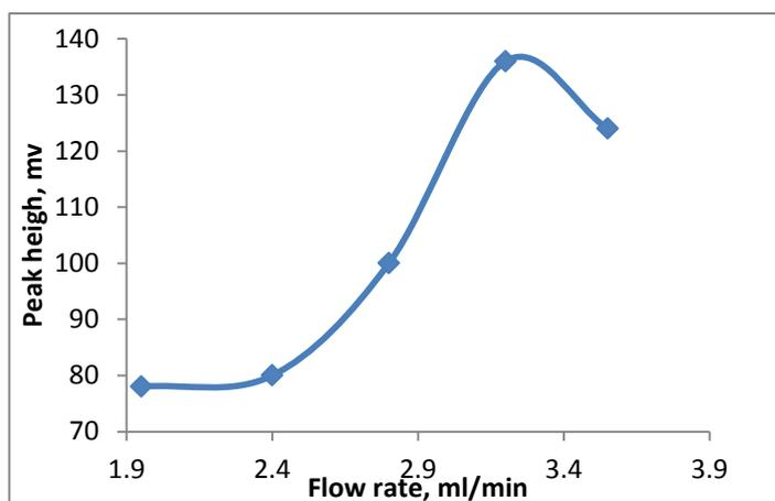
**Figure 7.** Effect of flow rate on analytical detection response.
