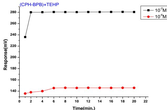
Figure 13. Response time of CPH-TEHP electrode.
