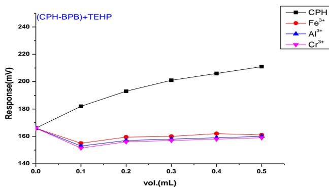
**Figure 17.** Selectivity for CPH-TEHP for tri-cations by match potential method.
