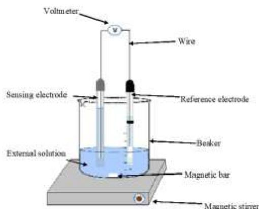
Figure 2. Diagram of ISE cell.
