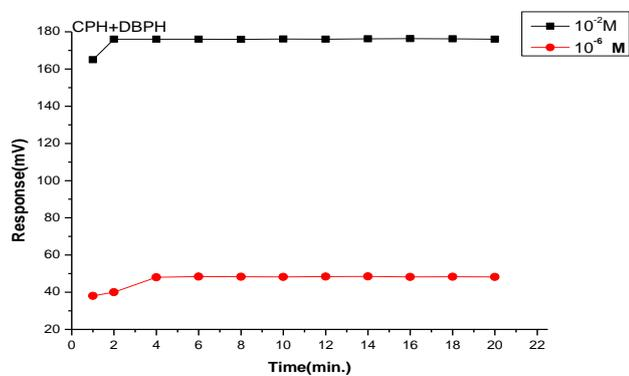
Figure 12. Response time of CPH-DBPH electrode.
