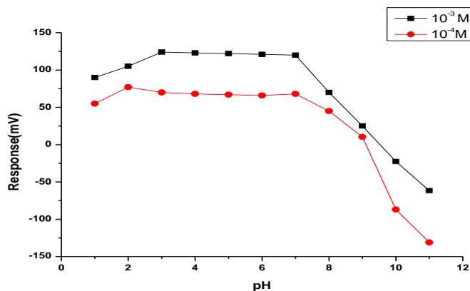
Figure 6. Effect of pH on the CPH-DBPH electrode response
