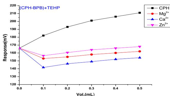
**Figure 16.** Selectivity for CPH-TEHP for di-cations by match potential method.
