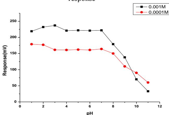
Figure 7. Effect of pH on the CPH-TEHP electrode response
