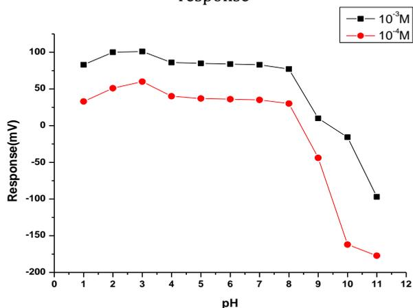
Figure 8. Effect of pH on the CPH-ONPOE electrode response
