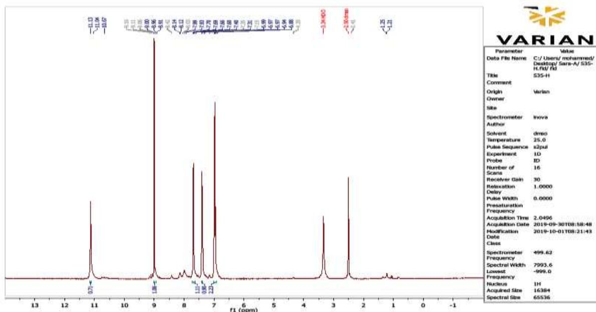
Figure 1. <sup>1</sup>H-NMR spectrum of 1, 2-hydroxy-5(4-(3-methyl-5-oxo-4,5-dihydro-1H-pyrazole-1-carbonyl)phenyl)diazanyl)benzylideneamino)quinolin-2(1H)-one (5).
