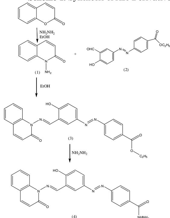
Scheme 2. Synthesis of acid hydrazide derivative from Quinoline.
