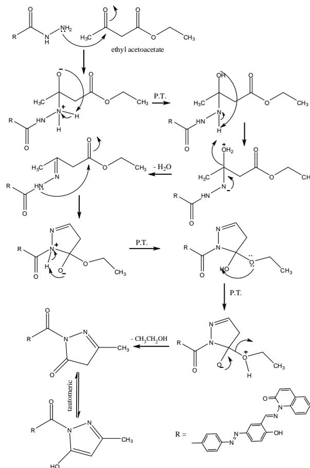
Scheme 4. Mechanisms of Synthesis of Pyrazoles derivative.
