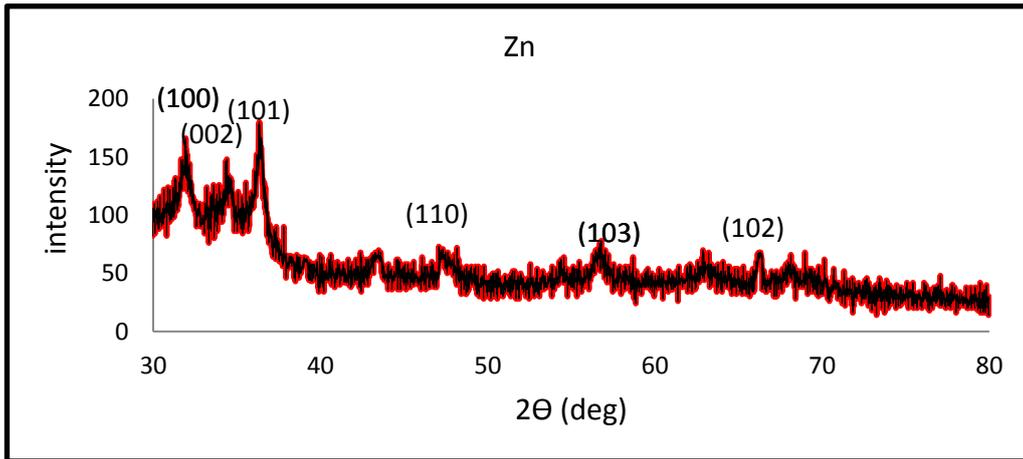
*Fig.(2) : XRD pattern of Zn target.*
