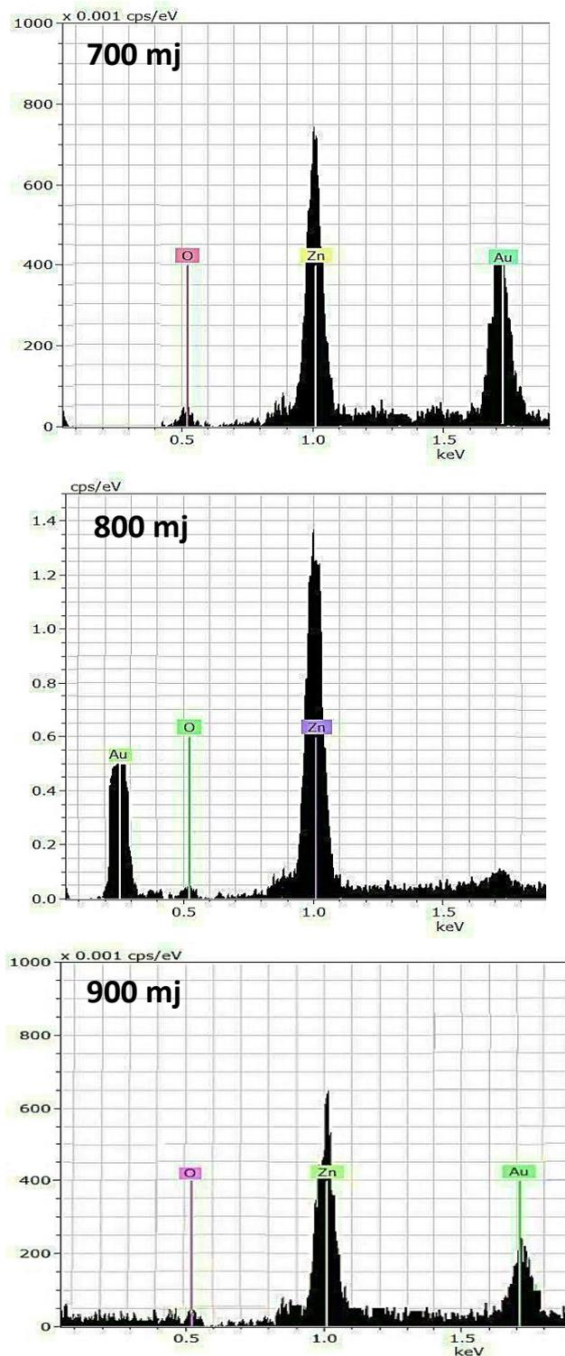
**Fig.(5): EDX of ZnO thin films deposited on a glass substrate at 85 C for ethanol with different laser energies (700, 800 and 900 mJ).**
