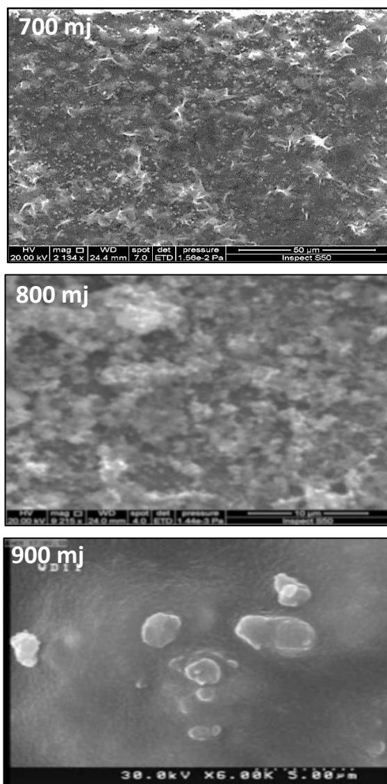
**Fig.(4): FESEM images of ZnO NPs prepared by pulsed laser ablation in ethanol with different energies (700, 800, 900 m.J) and pulses fixed (2000).**
