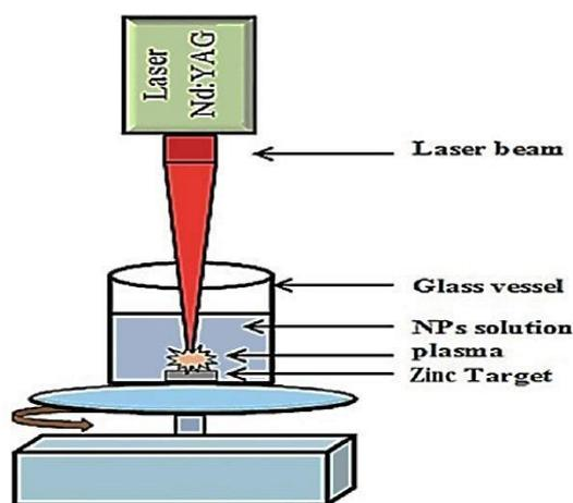
Fig.(1): Experimental setup of nanoparticle synthesis by PLA method.
