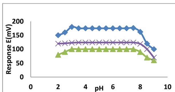
**Chart (3): Response of pH effect for (PCH) electrodes at concentration  $10^{-3}$  M of pilocarpine hydrochloride solution, ■  $E_1$ , ×  $E_2$ , ▲  $E_5$ .**
