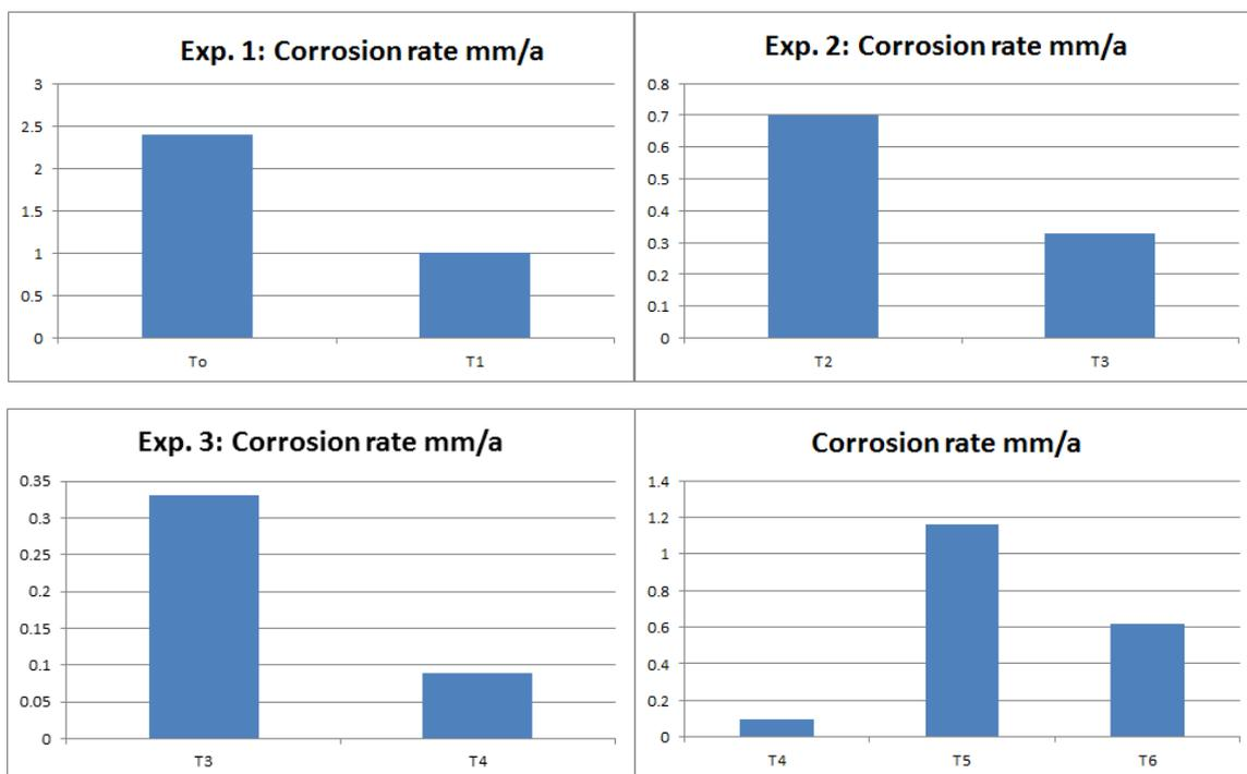
**Fig.(2):** Calculated corrosion rate found in the corrosion experiments of the studied mild steel rings according to Table (1).
